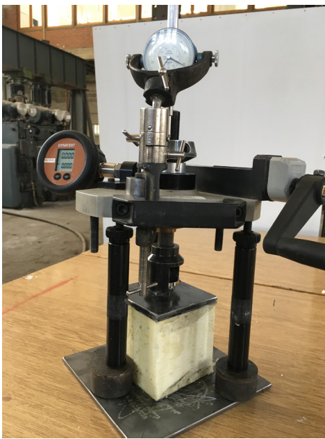
Figure 3. Specimen, left: before the test, right: after test (failure of panel core)
