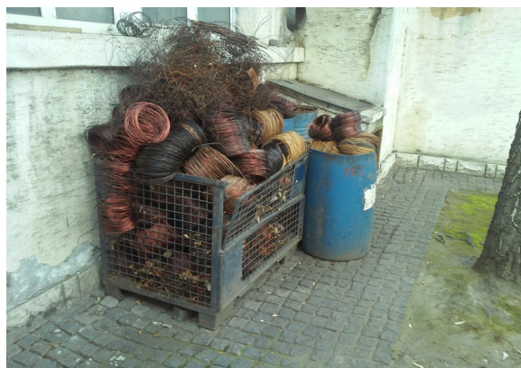
Figure 3. Collection of copper coils from scrapped electric motors of trams and trolleybuses in JKP GSP “Beograd”
