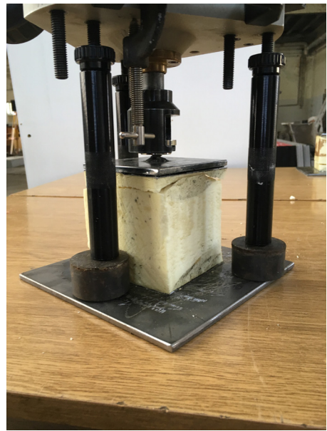
Figure 3. Specimen, left: before the test, right: after test (failure of panel core)
