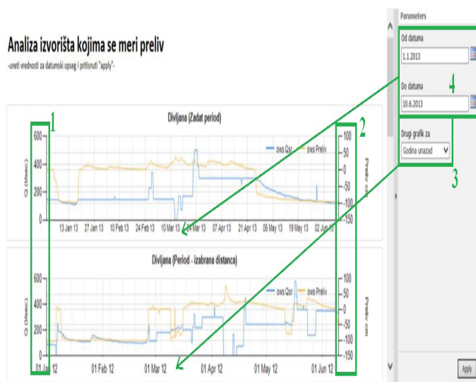
Figure 9: Analysis of springs where the overflow is measured- Source: Corporate portal JKP ,, NAISSUS,,
