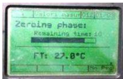
Figure 3. Zero calibration procedure of the Testo 350 M/XL analyzer.
