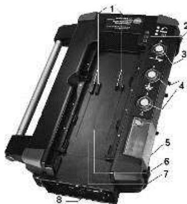
Figure 1. The analysis unit: 1 - electrical contacts; 2 - control LEDs; 3 - solid particle filter; 4 - filters for retaining particles from the aspirated air; 5 - condensate collection; 6 - analysis cells; 7 - integrated system for determining the gas velocity and pressure; 8 - connections.
