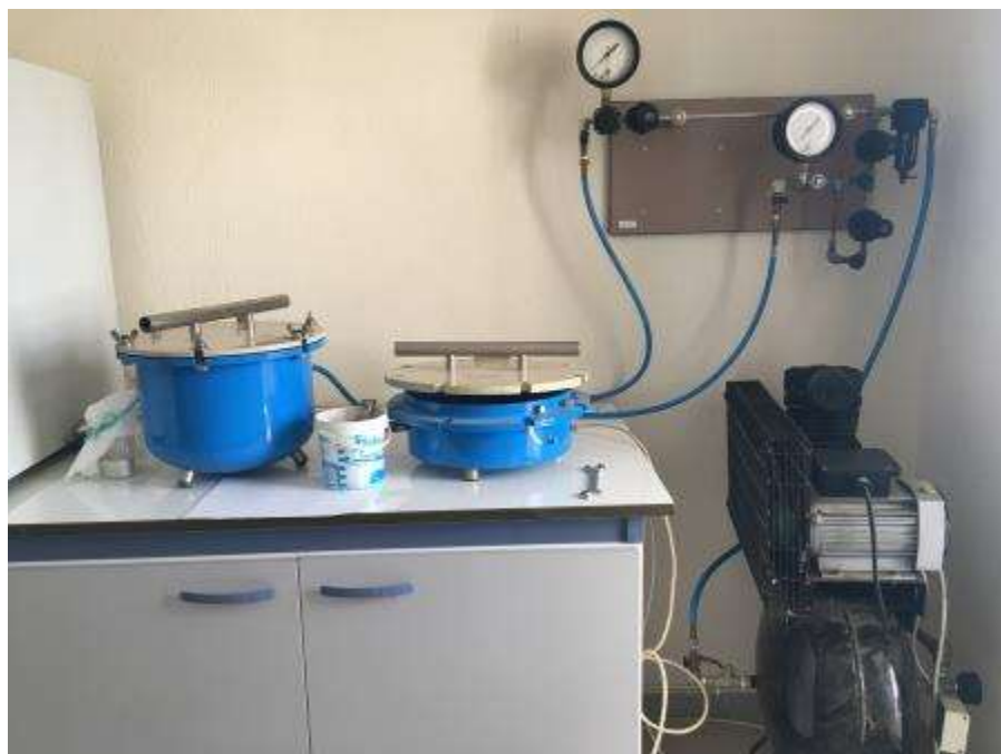
Figure 2. Pressure membrane extractor used to estimate the SMCCs.
