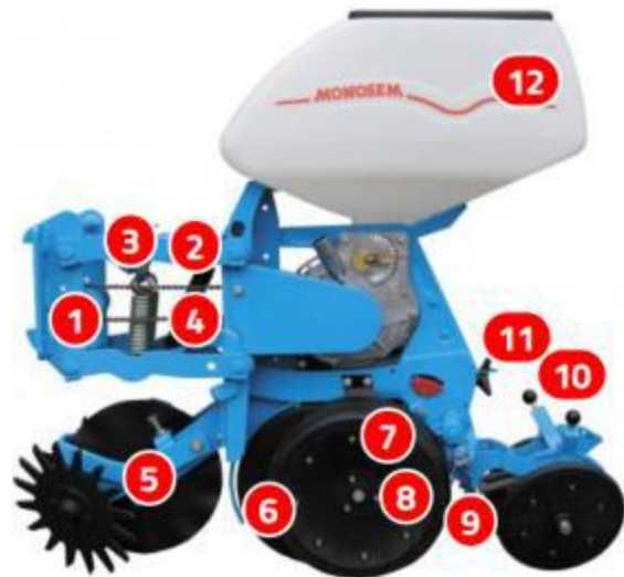
Fig. 2. Second type of seeding unit with more pressure on parallelogram linkage
