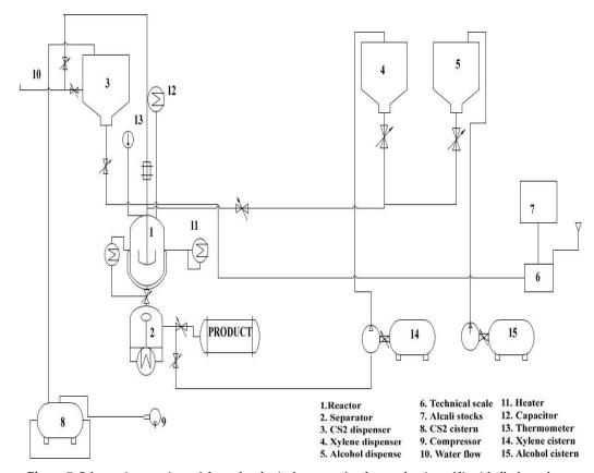
Figure 7. Schematic overview of the technological process for the production of liquid alkyl xanthate.
